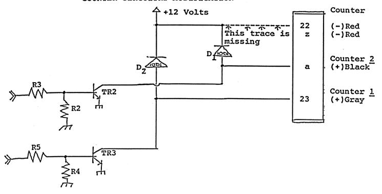
1.) You must add a wire from the cathode of D1, to the edge connector pin 22 and z to complete the circuit.
