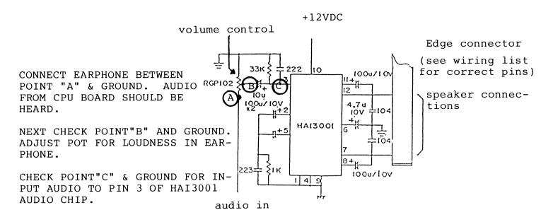
Also make sure Ground from +5VDC and Ground from +12VDC ARE TIED TOGETHER. IF GROUNDS ARE FLOATING, you could have audio problems.
